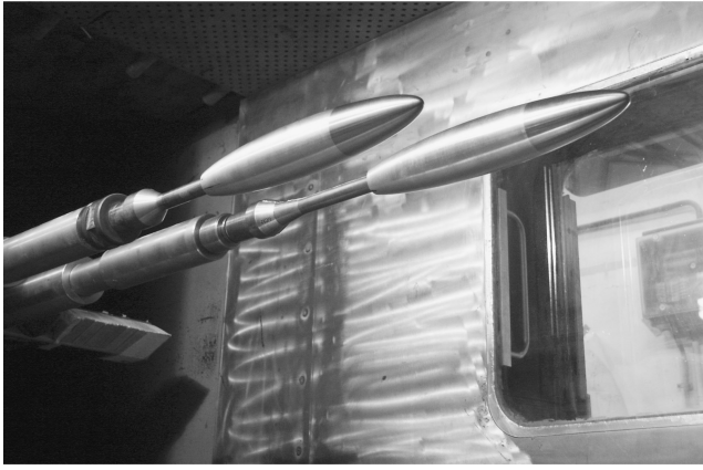
Fig. 1 Slender-body models in wind tunnel.
